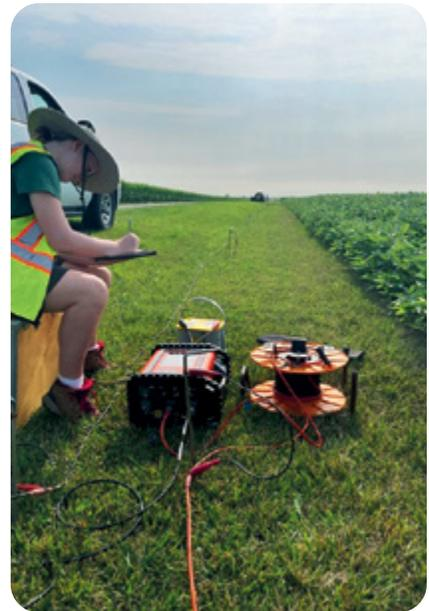
Carly Johnson taking a GPS point at the ERT station while waiting on the terameter to record its measurements.
