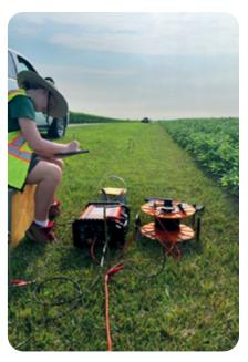
Carly Johnson taking a GPS point at the ERT station while waiting on the terameter to record its measurements.
